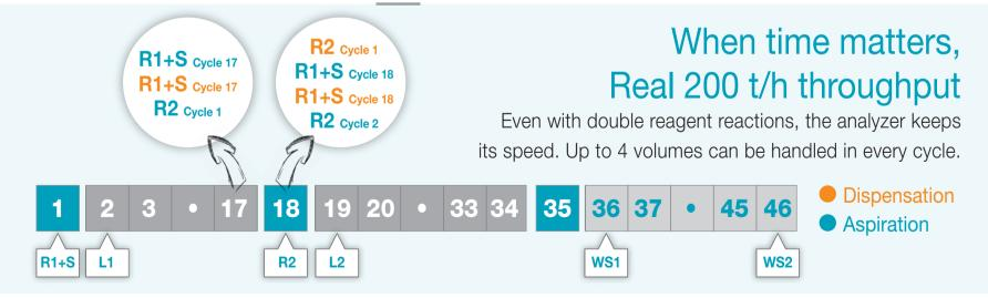
BA200 machine cycle sequence:R1 and sample are both dispensed in cycle 1, not requiring additional time for R1 pre thermo
